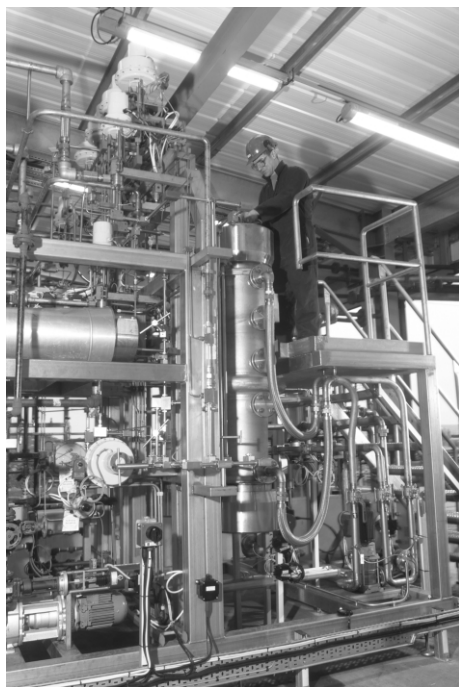
Fig. 6 Photograph of the reactor array in the Thomas Swan & Co. SCF reactions plant.
